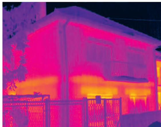
A family house with uninsulated massive brick walls. The house is not entirely heated; the thermal image clearly indicates the heated ground floor. The most noticeable heat losses occur in the zones of reinforced concrete ring beams and lintels. The window construction is inadequate, showing extensive heat loss especially at roller shutter boxes.
