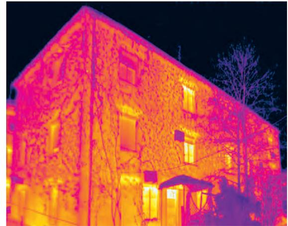
A residential *lamela* building with massive façade brick walls without thermal insulation. The thermal image shows heat losses evenly distributed through façade walls, particularly intense at lintel beams (and at walled-up ground floor opening). Some windows have been replaced with modern PVC with good thermal performance in contrast to original constructions characterized by noticeable heat loss.
