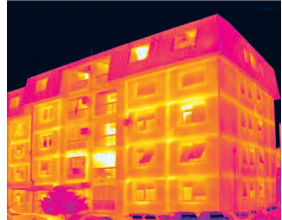
A residential building with façade walls built of prefabricated concrete panels. The thermal image shows heat loss at connections between panels and, less intensely, at the point of attachment to the final layer. Intense linear heat loss is characteristic at connections between terrace slabs and façade walls. Façade fenestration is of relatively poor quality and shows noticeable heat loss, particularly at roller shutter boxes.
