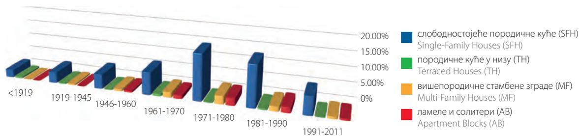
**Figure 12.** – National typology according to the TABULA – savings after the advanced level of improvement of building energy performance (% of current total energy consumption at national level)
