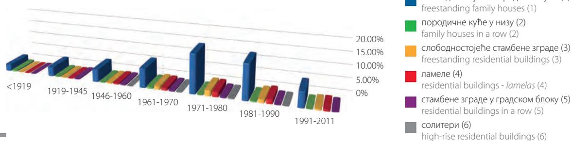
**Figure 11.** – National typology – savings after the advanced level of improvement of building energy performance (% of current total energy consumption at national level)
