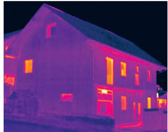
A family house with massive brick walls thermally insulated with a contact façade system. The thermal image reveals lower temperatures of the unheated attic wall, as well as heat losses at the points where cantilevered terraces penetrate the thermal envelope and at the eaves zone. The window and entrance door constructions are inadequate, showing noticeable heat loss.
